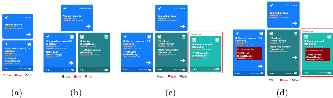
Figure 5.7: Step-by-Step Explanation: a sequence of screenshots of the user interface related to the step-by-step simulation of the inconsistency problem of Figure 5.6.
