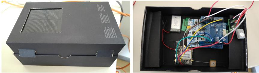
Figure 5.1. The cardboard case. On the right, the SwarmBike device inside the case
