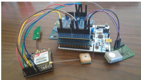
Figure 2: The prototype of the SwarmBike device: on the left the GPS/GPRS module, on the right the custom PCB with the CO sensor and the potentiostat, at the center the STM32 Nucleo board with the expansion shields
